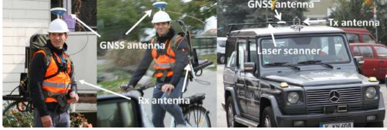
Figure 5.3: Antenna positions on the pedestrian, the cyclist, and the test vehicle.
