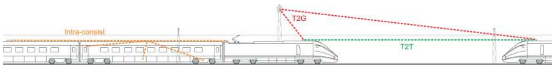
Figure 2.1: Railway communications: T2G, T2T, and intra-consist communication links.
